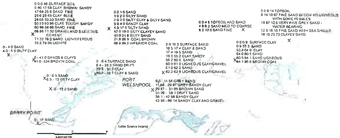
Figure 9. Location and log of upper sections of boreholes in the study area. Blue areas are wetlands (most are drained).
